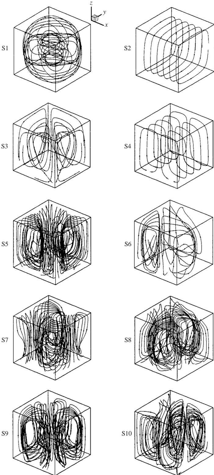
FIGURE 3. Flow trajectories of the steady convective patterns.
