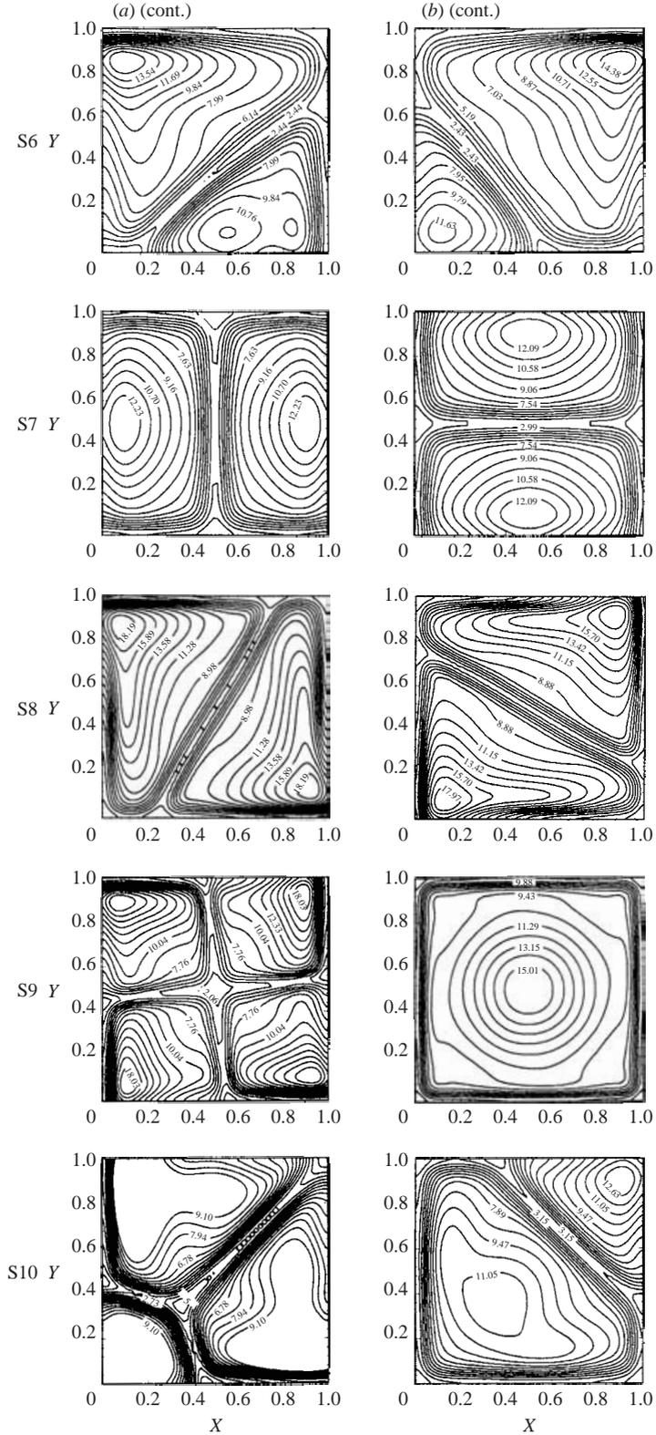
FIGURE 7. The distribution of the Nusselt number on (a) the top and (b) the bottom walls of the cubic cavity.
