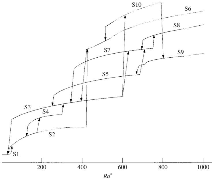
FIGURE 5. Schematic diagram of the flow transitions as a function of  $Ra^*$ . Solid (dotted) lines indicate steady (unsteady) solutions.
