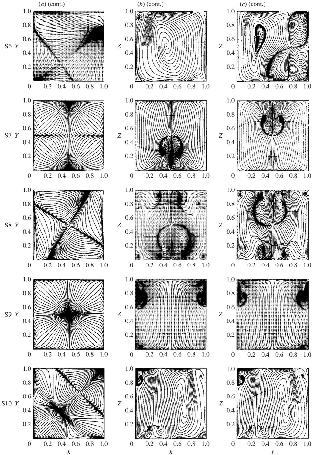
FIGURE 2. Steady-state convective patterns in the cubic cavity. (a) Projection of flow lines on the horizontal plane at  $Z = 0.9$ ; (b) projection of flow lines on the mid  $(x, z)$ -plane; (c) projection of flow lines on the mid  $(y, z)$ -plane.
