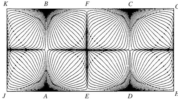
FIGURE 6. Projection of flow lines on the horizontal plane at  $Z = 0.9$  in a rectangular prism constructed from two adjacent cubes.
